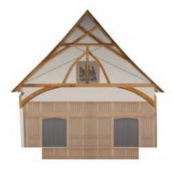
Proposed west elevational section cut forward of stage
